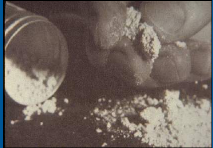
Photo of friable asbestos
