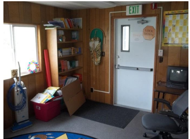
Culture Building (102T) – NE Corner of Classroom 5 Original floor covering has been hidden by wall-to-wall carpet. [Sheet vinyl flooring with 30% Chrysotile]
